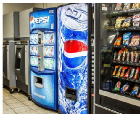
Vending machine GFCI protection cannot be factory installed within the appliance
