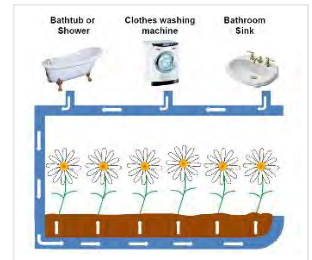
Greywater can be captured from your sinks, showers and washing machines and easily used for landscape irrigation.
